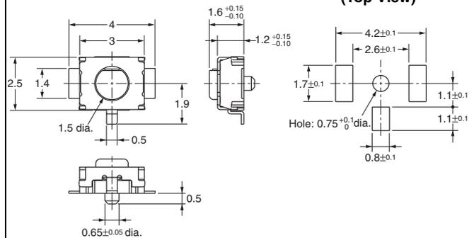
**Note:** Unless otherwise specified, a tolerance of  $\pm 0.2$  mm applies to all dimensions. No terminal numbers are indicated on the Switches.
