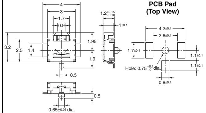
**Note:** Unless otherwise specified, a tolerance of  $\pm 0.2$  mm applies to all dimensions. No terminal numbers are indicated on the Switches.
