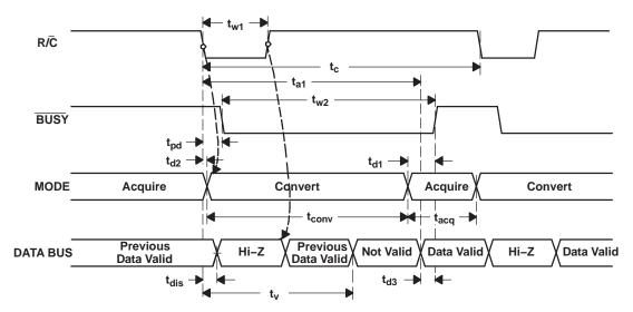
Figure 21. Conversion Timing with Outputs Enabled after Conversion ( $\overline{CS}$  Tied Low)
