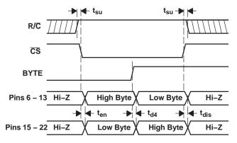
Figure 23. Using  $\overline{CS}$  and BYTE to Control Data Bus
