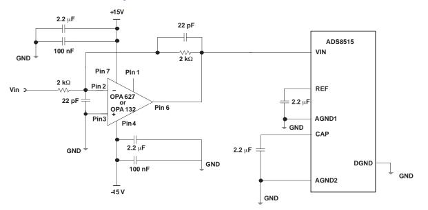
Figure 24. Typical Driving Circuit (±10 V, No Trim)
