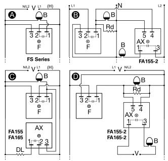
V = Voltage N = Neutral B = Beacon DL = Dummy Load for Constant Line Loading Rd =  $3.3 \text{ K}\Omega @ 5W$  for 120VAC;  $8.5 \text{ K}\Omega @ 5W$  for 230VAC F = Flasher (FS155-30T, FS155-30RF, FS165-30T) AX = Auxiliary Unit (FA155, FA155-2, FA165, FA156-2)
