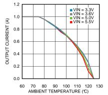
Thermal Derating V<sub>OUT</sub> = 3.3V, θ<sub>JA</sub> = 120°C/W
