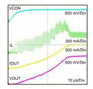
Figure 6. Startup behavior of current limit based softstart.
