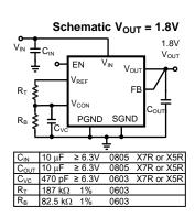
Output Ripple V<sub>OUT</sub> = 1.8V
