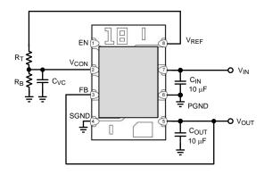
Figure 9. Typical Application Circuit
