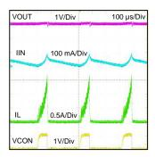
Figure 7. Hiccup behavior with persistent output short circuit.
