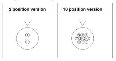
Note: The numbering of the contact is from the plug termination side.
