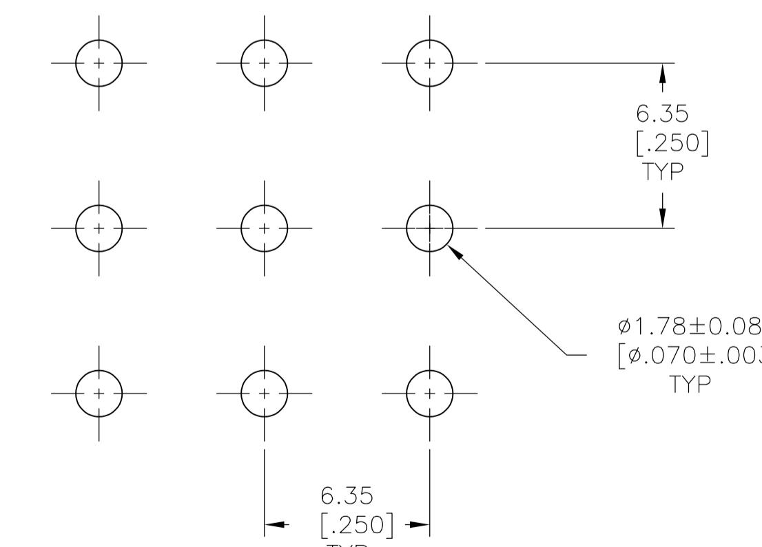
RECOMMENDED LAYOUT FOR 3.18 [.125] THICK PC BOARD
