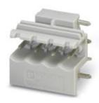
Header, Nominal current: 12 A, Rated voltage (III/2): 320 V, Number of positions: 4, Pitch: 5 mm, Mounting: Soldering
