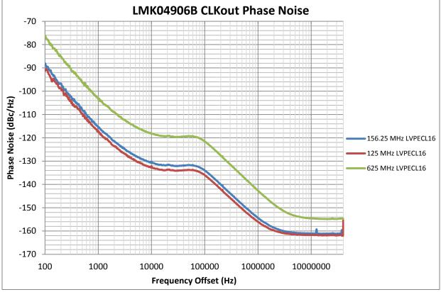
Figure 16: LMK04906B CLKout Phase Noise
