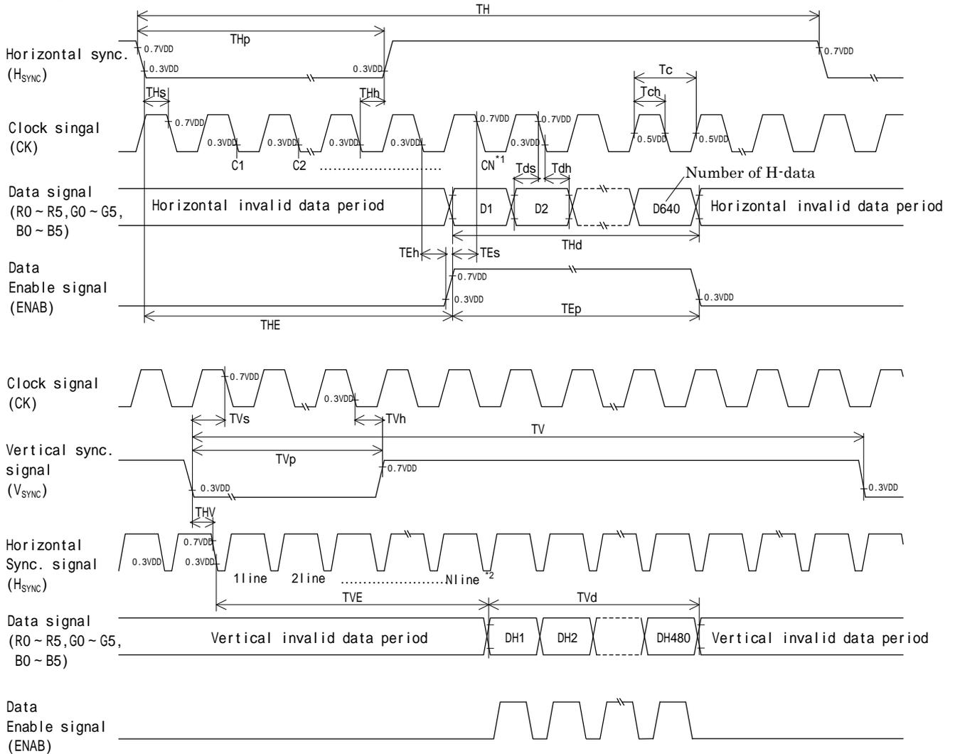
\*1 When ENAB is fixed at "Low", the horizontal display starts from the data of C144 (clock).
