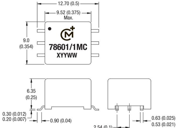
Unless otherwise stated all dimensions in mm (inches)  $\pm 0.25$  (0.01). All pins on a 2.54 (0.1) pitch and within  $\pm 0.25$  (0.01) of true position. Package Weight: 1.1g Typ.
