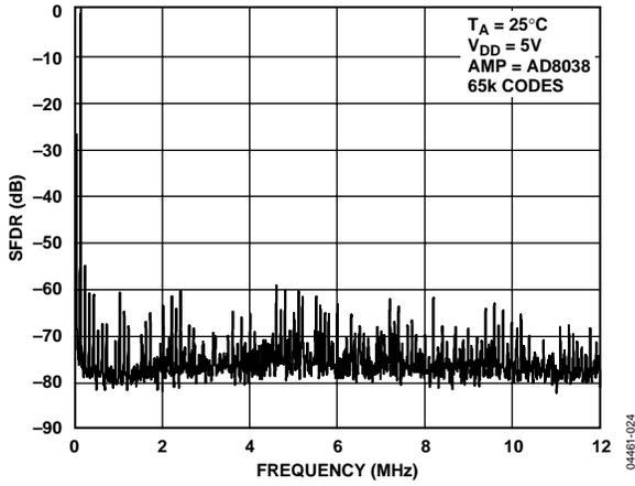
Figure 25. Wideband SFDR,  $f_{OUT} = 100$  kHz, Clock = 25 MHz
