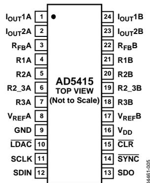
Figure 6. Pin Configuration
