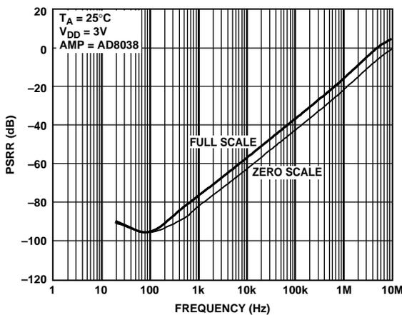
Figure 21. Power Supply Rejection Ratio vs. Frequency
