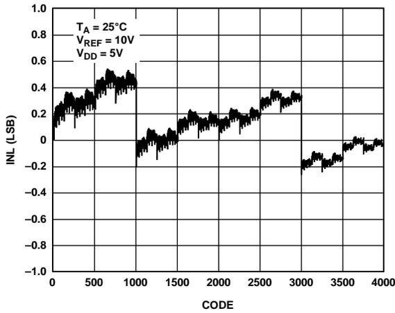
Figure 7. Integral Nonlinearity (INL) vs. Code (12-Bit DAC)
