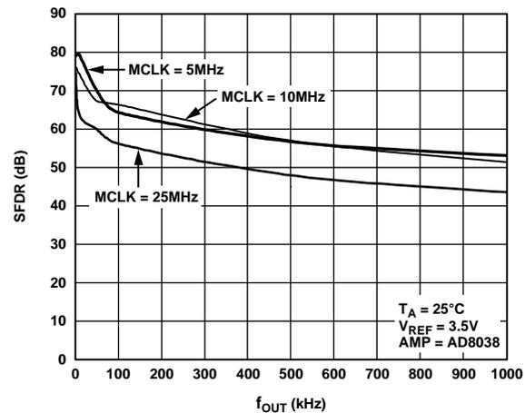
Figure 24. Wideband SFDR vs.  $f_{OUT}$  Frequency
