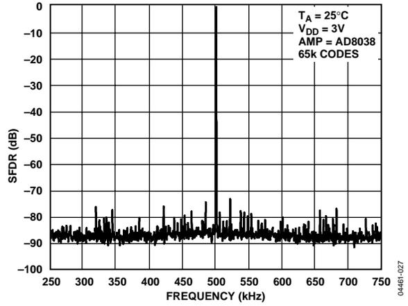
Figure 28. Narrow-Band Spectral Response,  $f_{OUT} = 500$  kHz, Clock = 25 MHz
