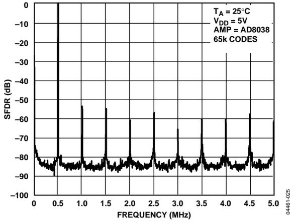
Figure 26. Wideband SFDR,  $f_{OUT} = 500$  kHz, Clock = 10 MHz
