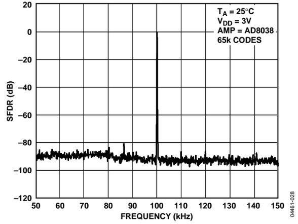
Figure 29. Narrow-Band SFDR,  $f_{OUT} = 100$  kHz, MCLK = 25 MHz
