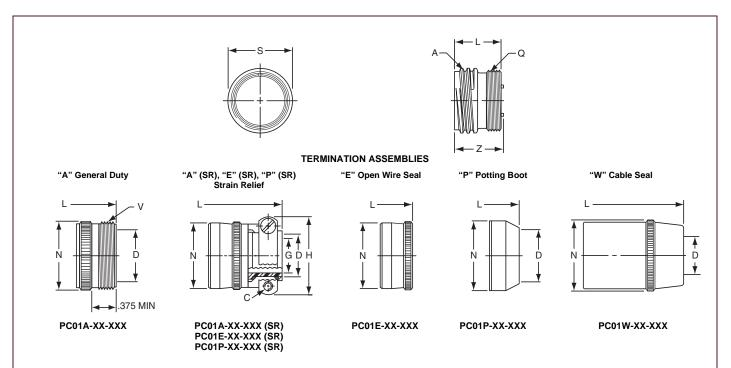
Note: This connector style is sometimes referred to as a cable connecting "plug". It does, however, mate with either a straight or 90 degree plug. To complete part number see how to order on page 61.
