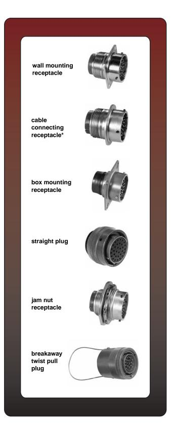
Amphenol<sup>®</sup> CE crimp type miniature connectors provide performance and versatility needed for applications demanding high reliability and crimp removable contacts. These crimp contacts are rear insertable/front release and are held in position by a nylon wafer retention system.
