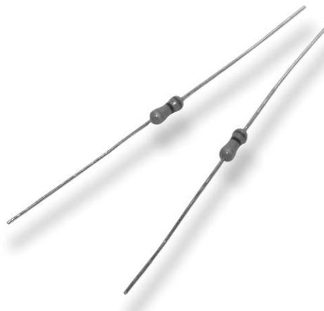
Metal glaze resistors are manufactured using thick film techniques. The ceramic slugs have the thick film applied, the film is fired and end caps are forced onto the slugs, the resistive element is spiralled to value and lead wires are welded onto the end caps. Four layers of coating are applied - the first being a phenolic resin, the other three being epoxy.
