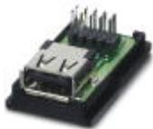
USB socket insert, 4-pos., socket USB type A on flat-ribbon cable terminal strip, pitch 2.54, for the Freenet system in the panel mounting frame, IP20 terminal outlet, 19" patch panel and service interface
