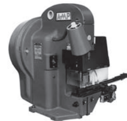
AMP-O-LECTRIC Bench Machine with Special Applicator
