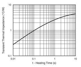
Fig. 6 - Typical Transient Thermal Impedance
