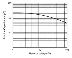
Fig. 5 - Typical Junction Capacitance Per Diode
