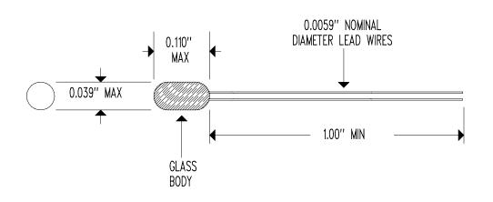
RESISTANCE @  $+25^{\circ}C$  = 1,000,000  $\Omega$  ± 5% RESISTANCE/TEMPERATURE CURVE = SEE GP105V8J REV.NONE R-T TABLE BETA " $\beta$ " (+25 TO +85°C) = 4,350°K NOMINAL DISSIPATION CONSTANT = 0.45 mW/°C NOMINAL (STILL AIR) THERMAL TIME CONSTANT = 0.20 SECONDS NOMINAL (STIRRED OIL) MAXIMUM TEMPERATURE RATING =  $+300^{\circ}C$
