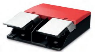
Standard OFF-ON Operation-Lift protective hinged cover up to activate pedal. Push pedal down to change contact state. Release pedal to return to original state. With IP67 Protection Rating (Temporary Submersion).
