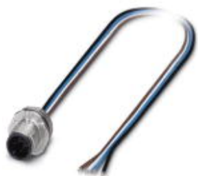
Sensor/actuator flush-type plug, 4-pos., M12 SPEEDCON, A-coded, front/screw mounting with M16 thread, with 1.1 m TPE litz wire, 4 x 0.34 mm 2
