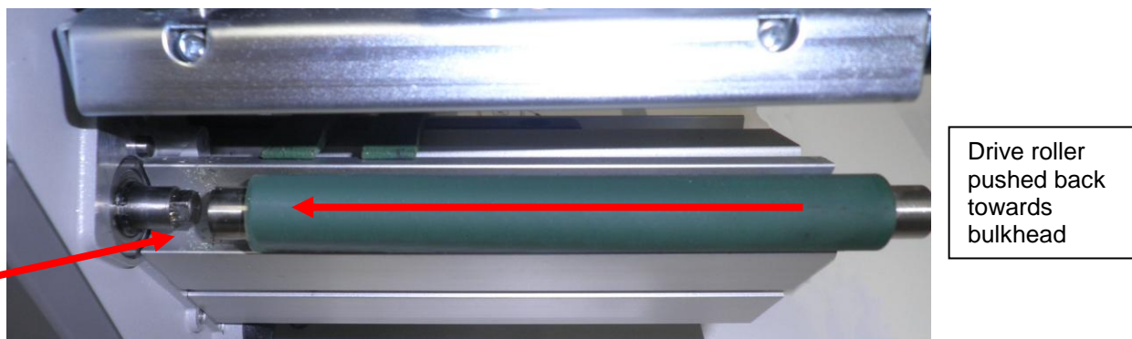
Figure 6 - Drive Roller removal
