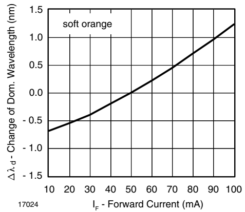
Fig. 18 - Change of Dominant Wavelength vs. Forward Current
