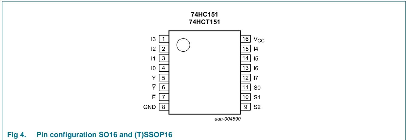
Fig 4. Pin configuration SO16 and (T)SSOP16
