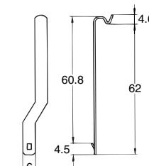
Use a PFC-A1 Mounting Bracket to mount the Surge Killer Unit to the PF113A Rail-mounted Socket.
