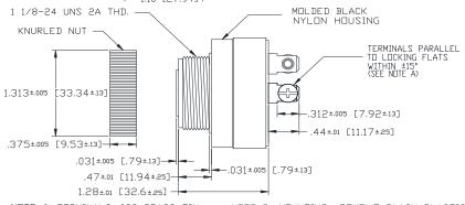
NOTE A: TERMINALS-032 BRASS TIN PLATED, TAPPED FOR #6-32 SCREW. TWO #6-32 NICKEL PLATED BRASS SCREWS INCLUDED. WILL ACCEPT 1/4" QUICK CONNECT.
