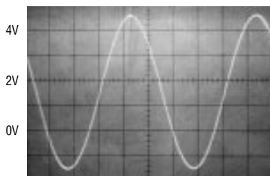
6V p-p INPUT, -1.5V TO 4.5V LT1413 • TA21
