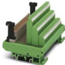
VARIOFACE module, for IEC 603/DIN 41612 connector, type F, 48-pos., z, b, d components mounted, with male connector, cable housing with screw interlock
