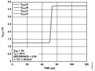
Figure 24. Settling Time
