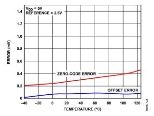
Figure 13. Zero-Code Error and Offset Error vs. Temperature
