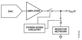
Figure 39. Output Stage During Power-Down
