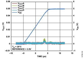
Figure 25. Power-On Reset to 0 V
