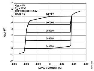
Figure 21. Source and Sink Capability at 5 V
