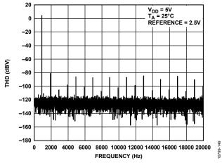
Figure 30. Total Harmonic Distortion at 1 kHz
