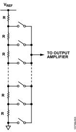
Figure 34. Resistor String Structure
