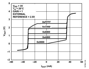
Figure 22. Source and Sink Capability at 3 V
