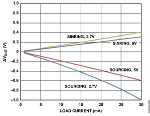
Figure 20. Headroom/Footroom vs. Load Current
