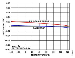
Figure 12. Gain Error and Full-Scale Error vs. Temperature
