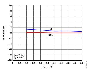
Figure 10. INL Error and DNL Error vs. V<sub>REF</sub>
