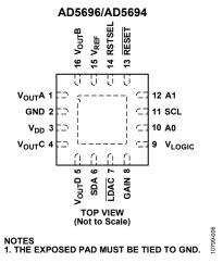
Figure 3. Pin Configuration, 16-Lead LFCSP
