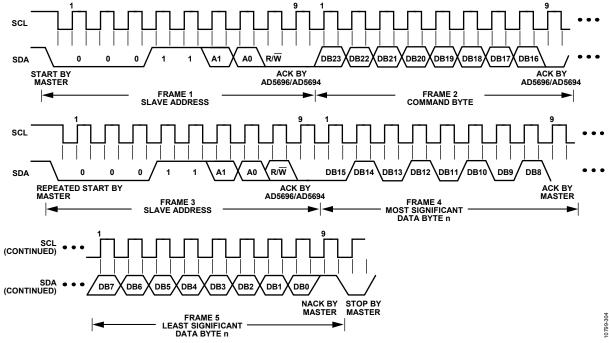
Figure 38. I<sup>2</sup>C Read Operation
