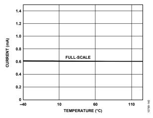
Figure 23. Supply Current vs. Temperature
