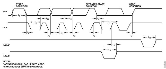
Figure 2. 2-Wire Serial Interface Timing Diagram
