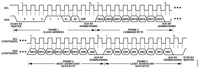
Figure 37. I<sup>2</sup>C Write Operation
