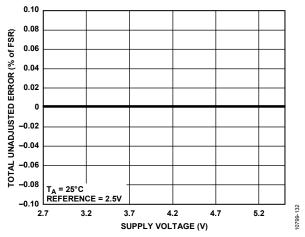
Figure 17. TUE vs. Supply Voltage, Gain = 1
