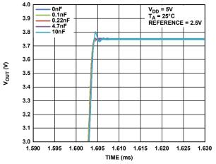
Figure 31. Settling Time vs. Capacitive Load
