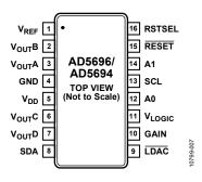
Figure 4. Pin Configuration, 16-Lead TSSOP
