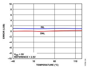
Figure 9. INL Error and DNL Error vs. Temperature
