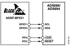
Figure 41. AD5696/AD5694 to ADSP-BF531 Interface
