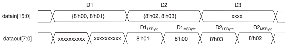
Figure 1–21. Byte Serializer Operation
