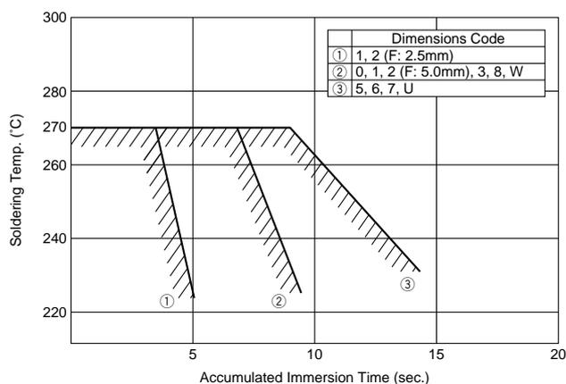
Perform soldering within tolerance range (shaded portion).
