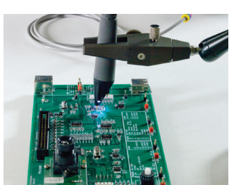
N2795A/96A comes with a headlight for better visibility while probing
