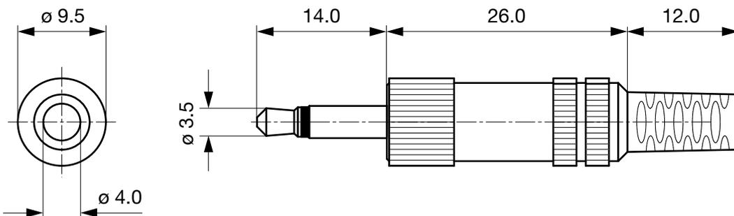
Cable diameter max. 4.0 mm
