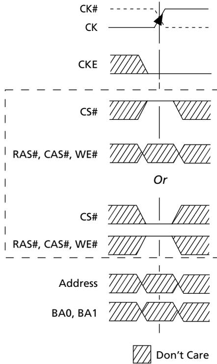
Figure 60: Power-Down Mode (Active or Precharge)
