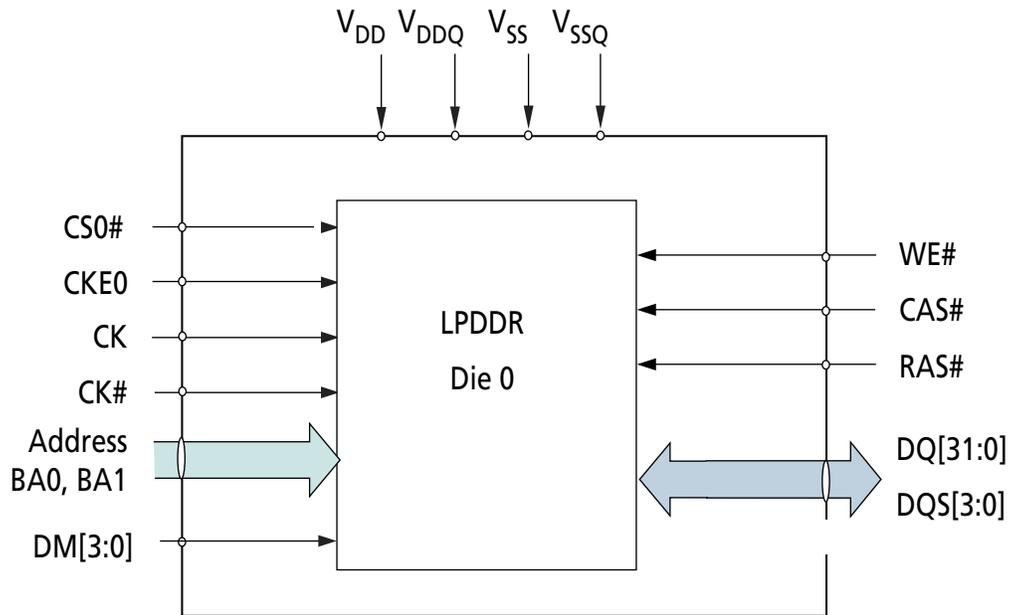
Figure 9: Dual Rank, Single Channel (2 Die) Package Block Diagram
