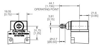
Figure 12. MICRO SWITCH™ LSX SERIES ADJUSTABLE SIDE PIN PLUNGER, HEAD CODE W • mm [in]
