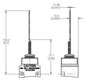
Figure 6. MICRO SWITCH™ LSX SERIES TOP ROTARY, **HEAD CODE B** • mm [in]
