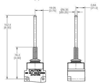
Figure 5. MICRO SWITCH™ LSX SERIES CAT WHISKER WOB-BLE, HEAD CODE K • mm [in]
