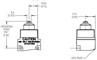
Figure 9. MICRO SWITCH™ LSX SERIES SIDE PLUNGER, **HEAD CODE E • mm [in]**
