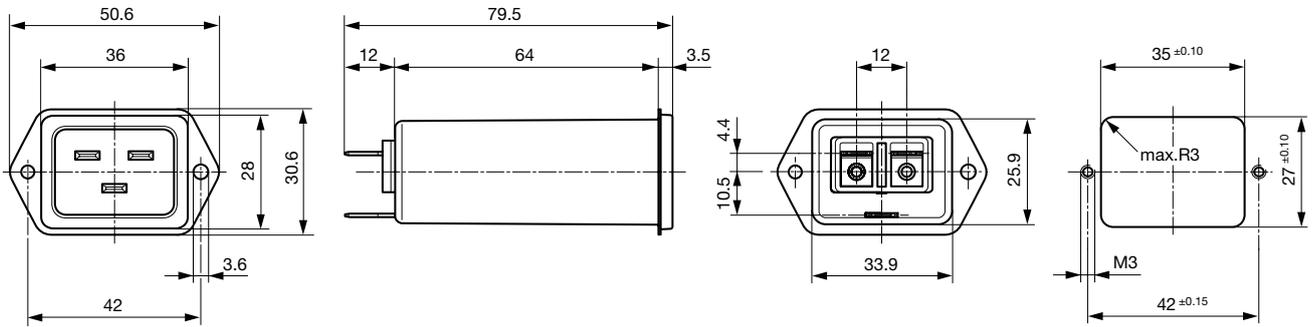
Rear side mounting with pre-formed, threaded holes for M3 screws
