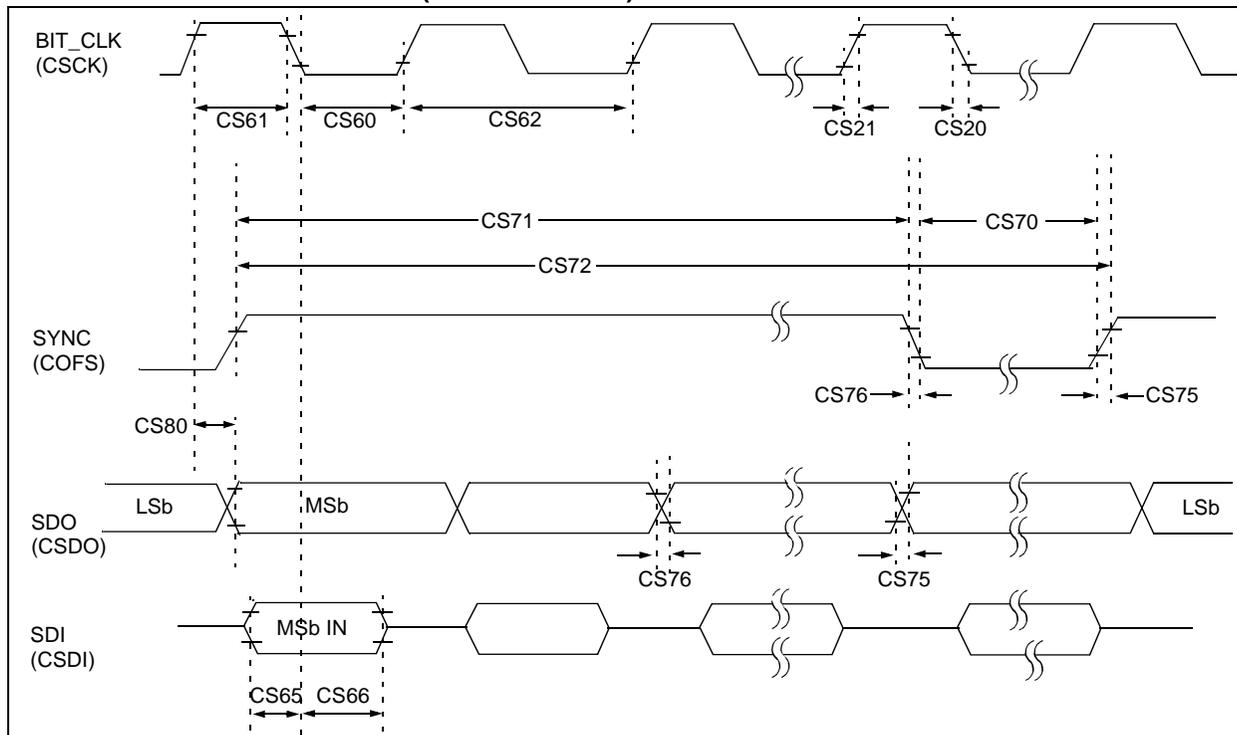
**TABLE 23-30: DCI MODULE (AC-LINK MODE) TIMING REQUIREMENTS**
