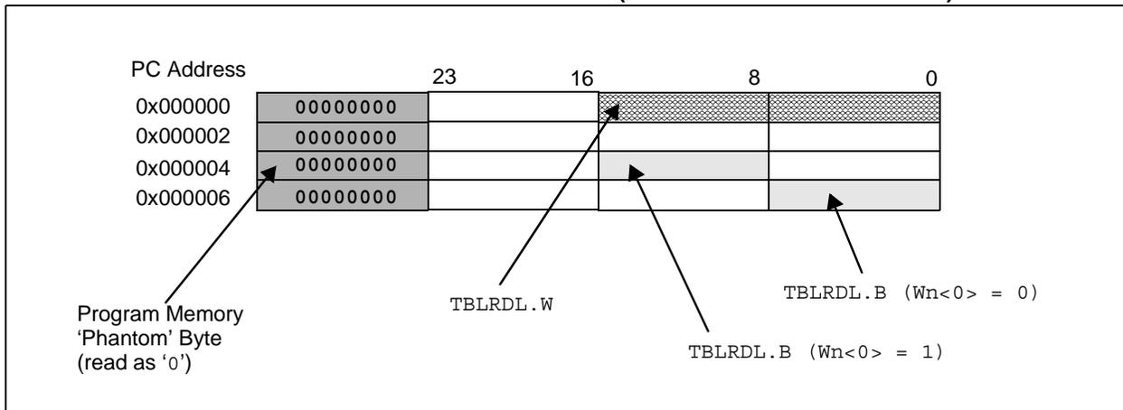
**FIGURE 3-5: PROGRAM DATA TABLE ACCESS (MOST SIGNIFICANT BYTE)**
