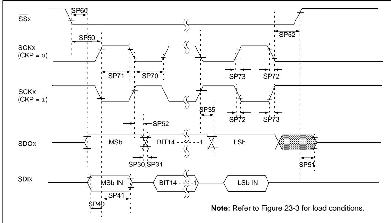
**TABLE 23-34: SPI MODULE SLAVE MODE (CKE = 1) TIMING REQUIREMENTS**
