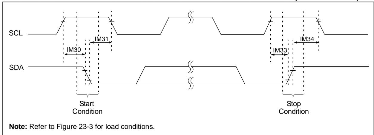
**FIGURE 23-19: I<sup>2</sup>C™ BUS DATA TIMING CHARACTERISTICS (MASTER MODE)**
