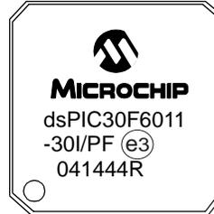
80-Lead TQFP (14x14x1mm)
