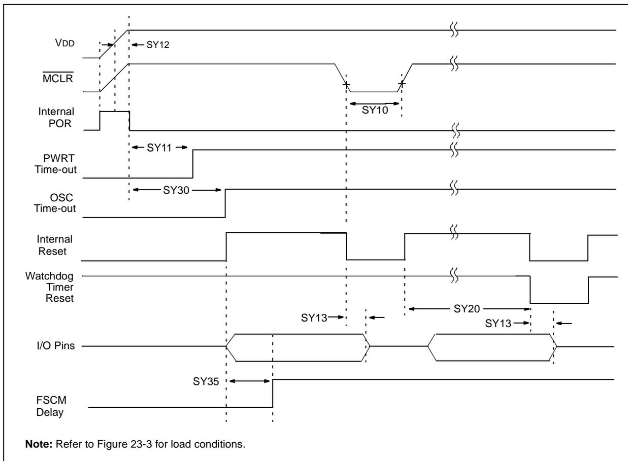
**TABLE 23-21: RESET, WATCHDOG TIMER, OSCILLATOR START-UP TIMER, POWER-UP TIMER AND BROWN-OUT RESET TIMING REQUIREMENTS**
