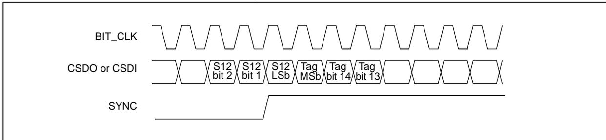
**FIGURE 18-4: I<sup>2</sup>S INTERFACE FRAME SYNC TIMING**
