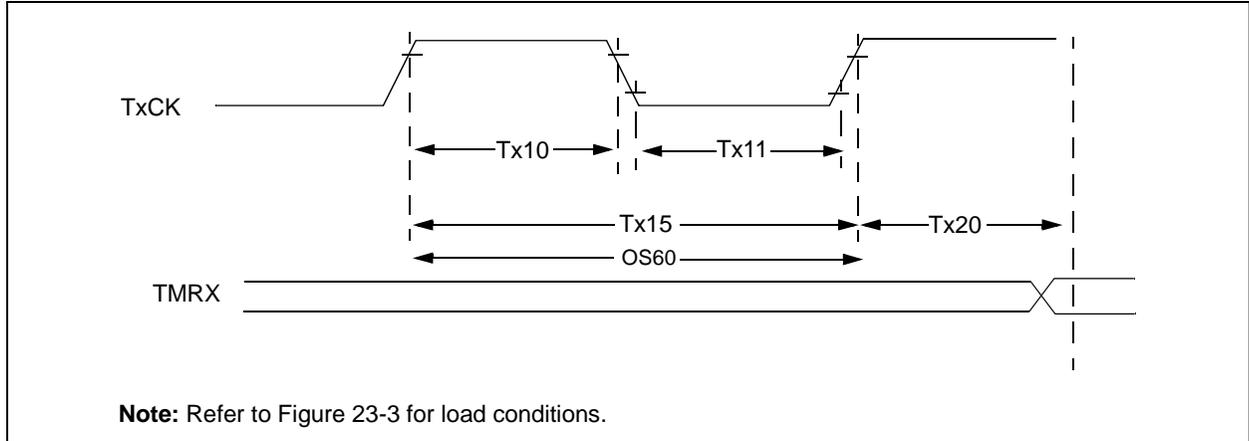
**TABLE 23-23: TYPE A TIMER (TIMER1) EXTERNAL CLOCK TIMING REQUIREMENTS<sup>(1)</sup>**
