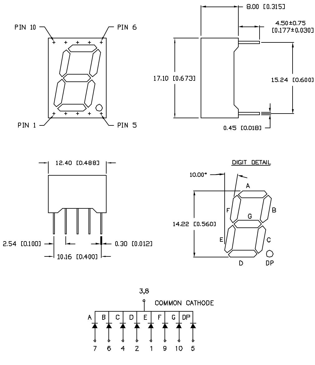
UNLESS OTHERWISE SPECIFIED TOLERANCE IS ±.25mm (±0.010")
