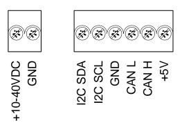
I2C is a short-distance intra-device bus that can be used to add capabilities such as an ADC (for analog measurement) or digital inputs and outputs.
