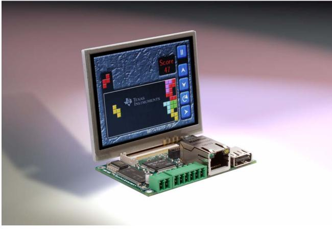
Figure 1-1. Intelligent Display Module Single-Board Computer
