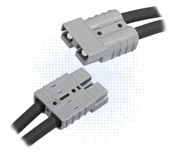
Based off the design pioneered by Anderson in 1953, the two pole SB<sup>®</sup> connectors set the standard for DC power distribution and battery connections. SB<sup>®</sup>50 connectors feature a one piece plastic housing using stainless steel springs to hold low resistance contacts in place. Wires sizes from #16 (1.5 mm<sup>2</sup>) to #6 (13.3 mm<sup>2</sup>) are held in the smallest of the SB<sup>®</sup> series housings.
