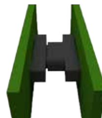
Straight receptacle to straight plug
