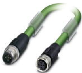
Bus system cable, INTERBUS, 5-position, PUR halogen-free, green RAL 6017, shielded, Plug straight M12, B-coded, on Socket straight M12, B-coded, cable length: 1.5 m
