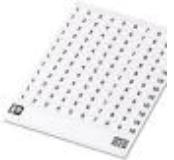
Marker card, Card, white, unlabeled, can be labeled with: Marker pen, Mounting type: Adhesive, for terminal block width: 6.2 mm, Lettering field: 6.2 x 3.8 mm
