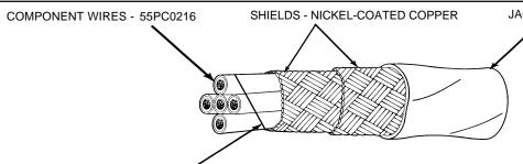
JACKET - RADIATION-CROSSLINKED, MODIFIED ETFE
