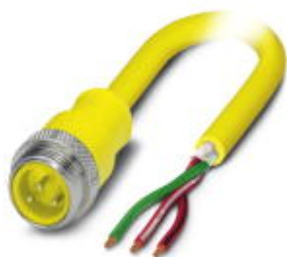
Sensor/actuator cable, 3-position, PVC, yellow, Plug straight 7/8"-16UNF, A-coded, on free cable end, cable length: 4 m
