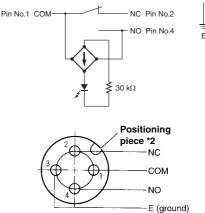
\*1. "Lit when not actuated" means that when the actuator is in the free position, the indicator is lit, and when the actuator is turned or pushed and the contact comes into contact with the NO side the indicator turns OFF
