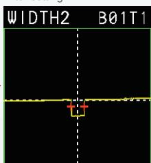
Lost part on a profile due to insufficient amount of light received
