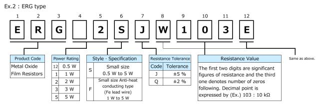
The above example 2 shows a small metal oxide film resistor, 2 W power rating, resistance value of 10 kΩ, tolerance ±5 %, and package of radial taping.
