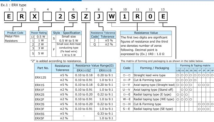
The above example 1 shows a small metal film resistor, 2 W power rating, resistance value of 1.0  $\Omega$ , tolerance ±5 %, and package of radial taping.
