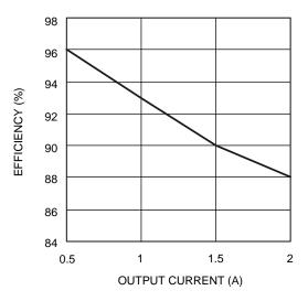
Figure 2. Efficiency vs Output Current  $(V_{IN} = 5 V)$
