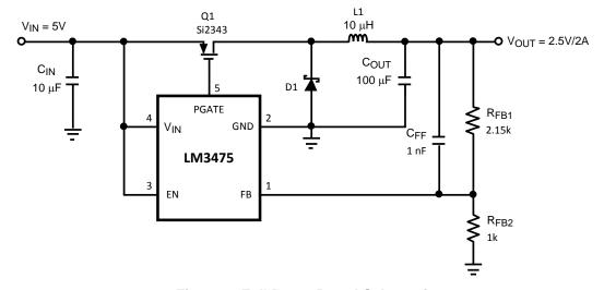
Figure 1. Full Demo Board Schematic
