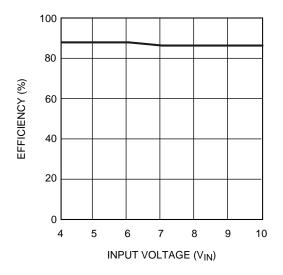
Figure 3. Efficiency vs Input Voltage ( $I_{out} = 2A$ )
