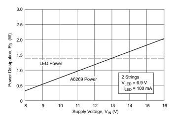
Figure 5. Power Dissipation versus Supply Voltage
