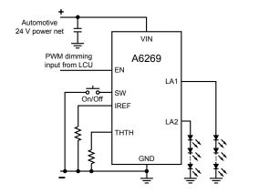
Figure 10. Typical applications using SW and EN together
