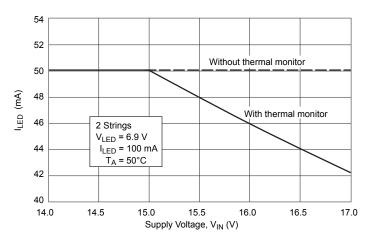
Figure 6. LED current versus Supply Voltage
