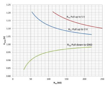
Figure 3b. Typical Resistor Values to Set Voltage on THTH Pin.
