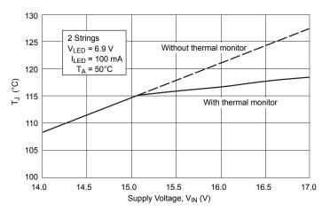
Figure 7. Junction Temperature versus Supply Voltage
