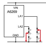
A. Any LED cathode short to ground. Current remains regulated in non-shorted LEDs. Matching may be affected
