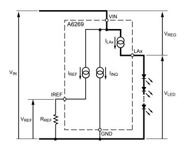
Figure 4. Internal power dissipation sources.
