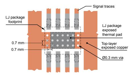
Figure 8. Suggested PCB layout for thermal optimization (maximum available bottom-layer copper recommended)
