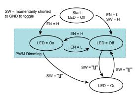
Figure 11. State diagram when both SW and EN are used
