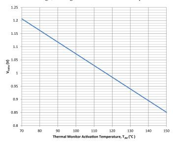
Figure 3a. Relationship between  $T_{\text{JM}}$  and  $V_{\text{THTH}}$
