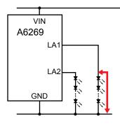
B. Any LAx output short to ground. Shorted output is disabled. Other outputs remain active.
