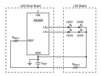
Figure 12. Application Circuit for Binning – Current-setting resistor ( $R_{\text{REF2}}$ ) can be placed on LED board for different bins of LEDs
