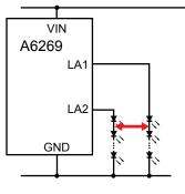
D. Short between LEDs in different strings. Current remains regulated. Current is summed and shared by affected strings. Intensity match dependent on voltage binning.
