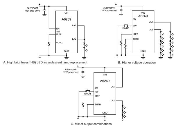
Figure 9. Typical applications with various supply and output options.
