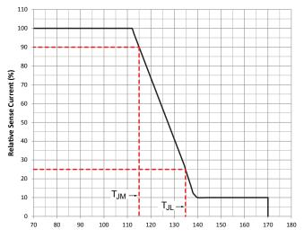
Figure 2. Temperature monitor current reduction.
