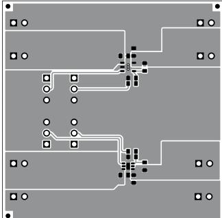
Figure 5. Top Assembly Layer
