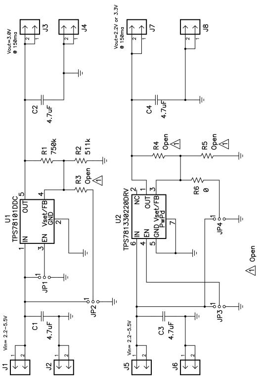
Figure 9. TPS78101EVM Schematic
