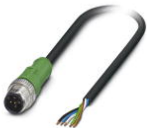
Sensor/actuator cable, 5-position, PVC, black RAL 9005, Plug straight M12, A - standard, on free cable end, cable length: 2 m
